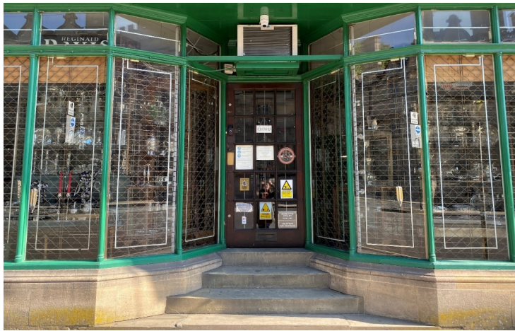
Figure 48: Shopfront with discreet, internal security shutters that allow visibility into the premises (not in Reading) (Source: RBC Planning).
