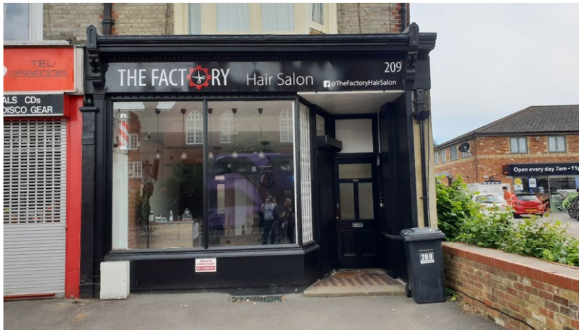
Figure 3837: Good example of signage, on Oxford Road. Note a well detailed timber glazed black shopfront. This is also a good example of incorporating both a ground floor retail entrance and entrance to access residential properties on the first floor. (Source: RBC Planning).
